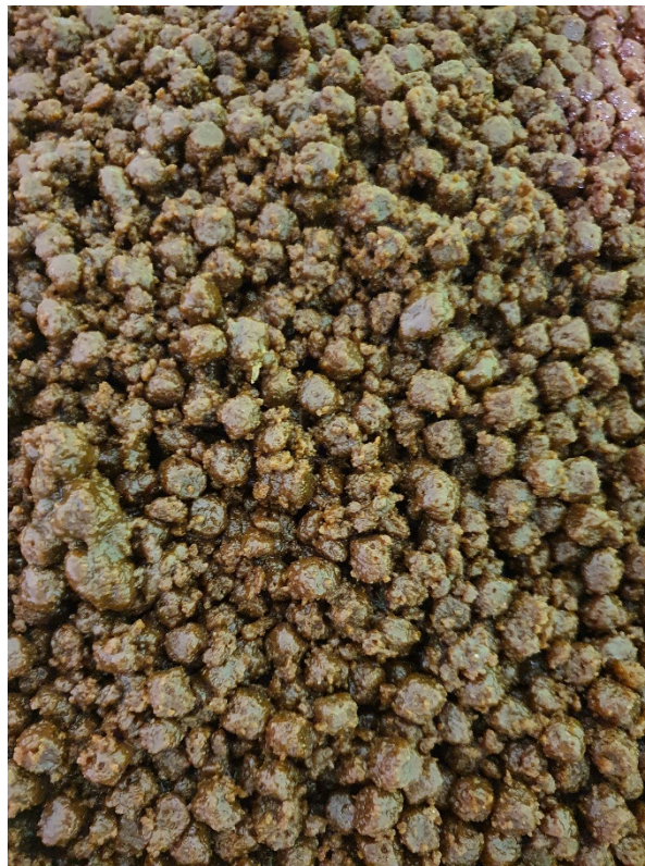
Figure 16: Degraded pellets after seven rounds of transport in the pneumatic conveying rig, the size of the pellets is reduced, and pellet debris are apparent.
