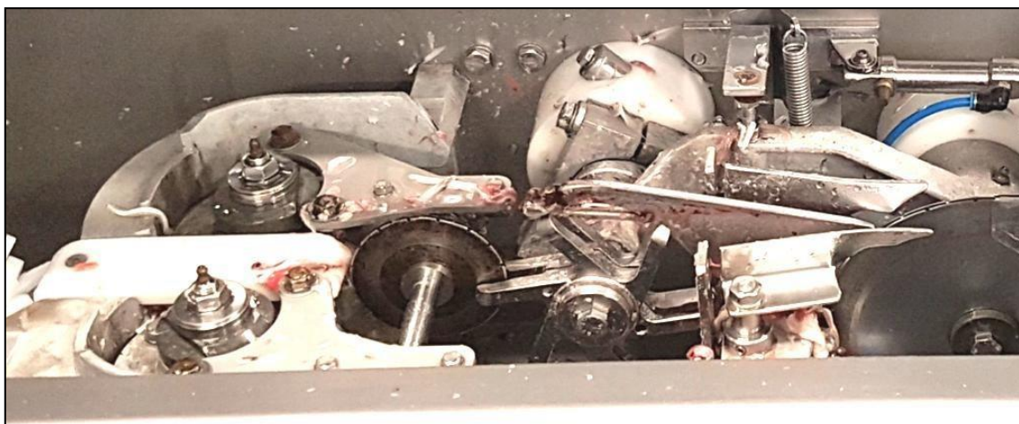
Additional belly cut and new gutting wheel
