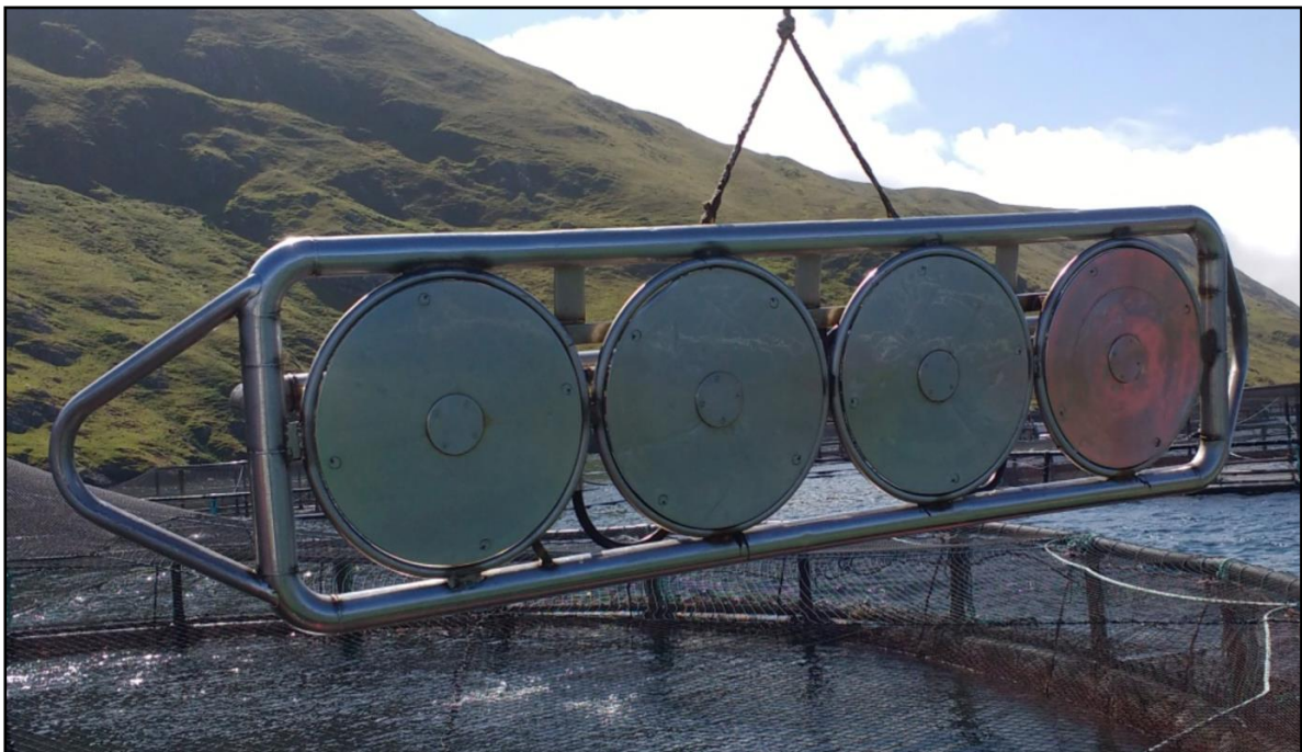
Figure 2.2.4-1. Example of a net cleaning rig from AKVA with 4 cleaning heads. Photograph courtesy of N. Ribeiro, with permission.
