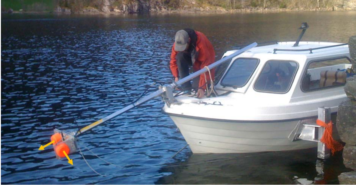
Figure 1 Vessel with rigging of the transducers with pole in lifted position, here rigged with one transducer pointing downward and one pointing to port (standard setting during application). In operation the pole would be lowered so that its angle with the water was 90 degrees. Arrows indicate transmission directions of transducers.
