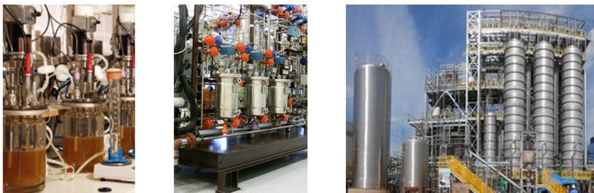
Figure 16. Different fermenting set-ups from lab-scale, pilot-scale and at the industrial scale (left to right). Source: SINTEF Materials and Chemistry and www.amyris.com .
