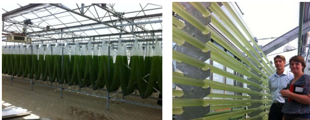
Fig. 21. ProAlgae visits at industria production sites. Left: The pilot production unit at NOVAgreen is a serial V-bag system, where each module holds 4 500 L of continuous culture. Right: The production units at Salata GmbH are glass tube vertical tubular PBR provided and installed by IGV. Photo: H. Kleivdal
