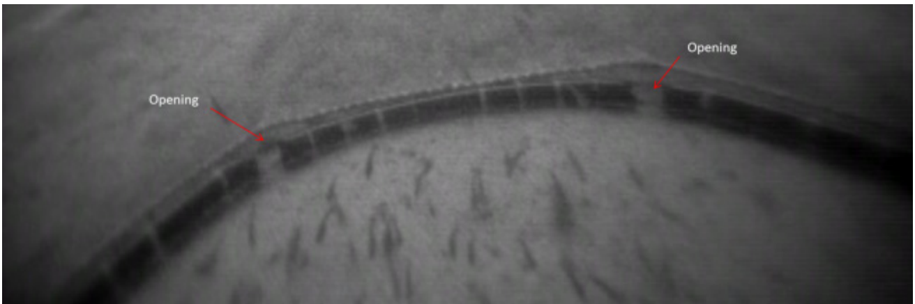
Figure 6. Underwater photograph showing the unintentional open spaces between the mid section and the side sections of the gear.
