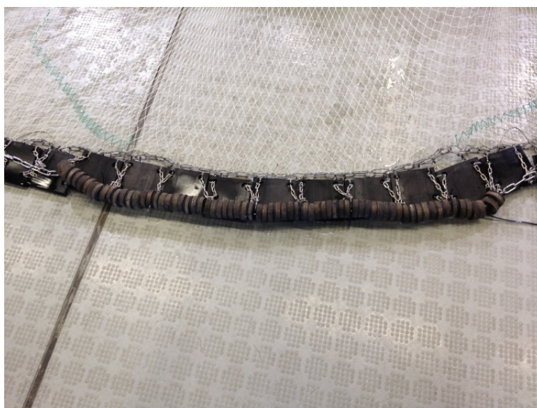
Figure 18. Center section of the gear chain filled with 200 mm (full-scale dimension) spacers in MP2, cases 5l- and 5m.
