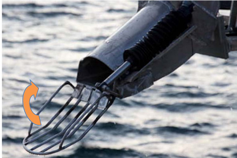
Figure 4 The modified extension on the ROV suction tube designed for collection of scallops. The steel rake is designed to pick up the scallop and tip upwards (as shown by the orange arrow) to bring the scallop into the range of the suction from the tube.
