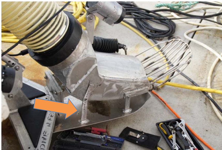
Figure 8 The modified collection system (rake) with a skid attached underneath (shown by orange arrow) to avoid the ROV nose diving into the sand.
