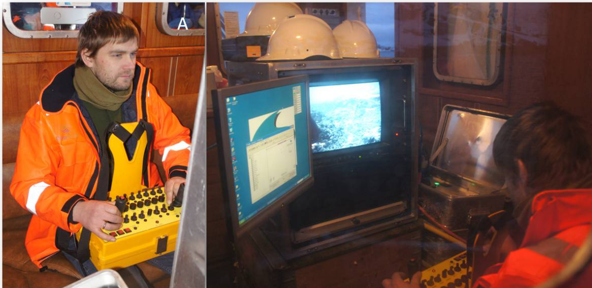
Figure 5 The ROV driver (Tor Andreassen) at the controls of the ROV in the wheelhouse of the R.V. Annabelle and the control monitors used during dive operations.
