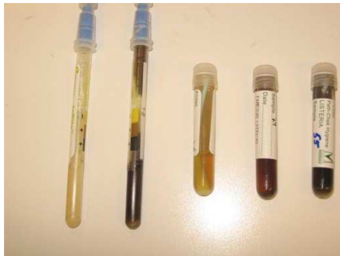
Figure 1 Rapid cultivation methods Includes swabs for sampling and tubes with growth medium into which the swab is transferred after sampling. The presence of listeria in the sample will cause an enzymatic colour reaction that can be observed visually following an incubation period of 24-48 hours at 30 or 37°C. Potentially listeria-positive samples (no. 2, 4 and 5 from the left) develop a colour change from straw-coloured to brown/black, while listeria-negative samples will should not change colour.
