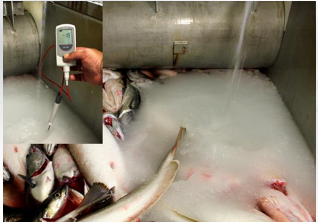
Measuring temperature in bleeding tank with ice slurry
