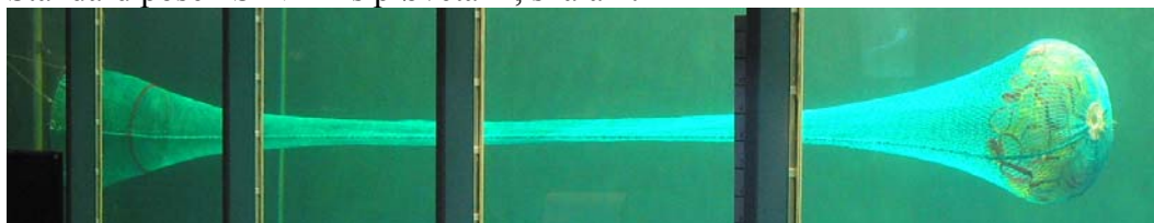
Standard pose i SINTEFs prøvetank, skala 1:2
